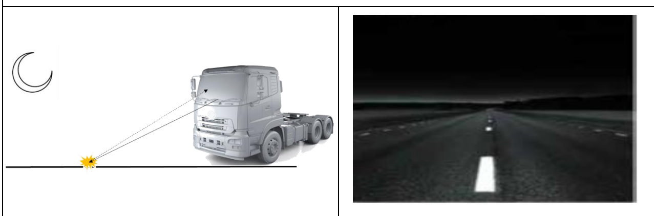
Figure 15.4 Night Visibility of Road Marking
