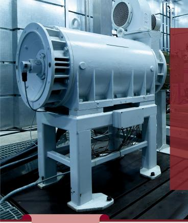
Engine Test Cell (ETC) facility at ICAT caters to the certification and development testing of engines as per National & International Standards. This includes emission testing of engines from automotive vehicles (with GVW above 3.5 tonnes) & Off-road engines (CEV's, Tractors, Power Tillers and Gensets). Also power testing of 2/3/4 wheelers is carried out in ETC.
