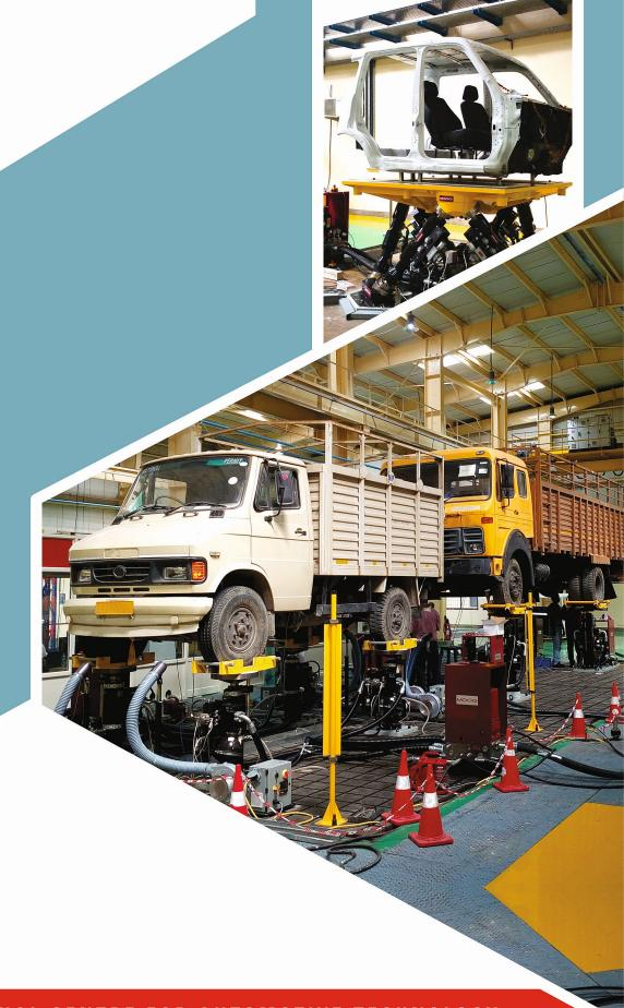
Fatigue Test Lab at ICAT is modern, state-of-the-art testing facility supporting automakers and suppliers for development and validation of various Structural Components, Sub-assemblies and vehicles. To ascertain the life of the product, lab is having expertise in the collection of road load data as per real world usage pattern, designing test specifications for accelerated duty cycle and execution of tests for customer correlation.
